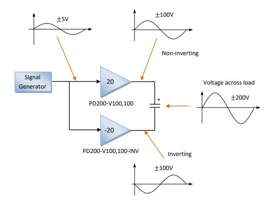
Figure 5. Bridge mode configuration for obtaining  $\pm 200V$
