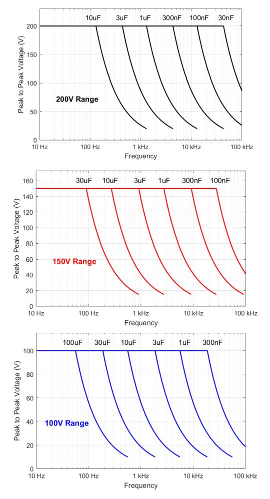
Figure 2. Maximum peak-to-peak voltage versus frequency and load capacitance
