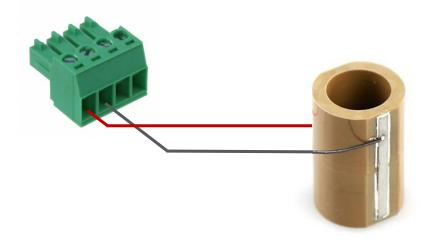
Bender actuators can be driven with a single bias voltage, for example 200 V, or a bipolar bias voltage, for example  $\pm 100$  V. The  $\pm 100$  V bipolar configuration is shown below.
