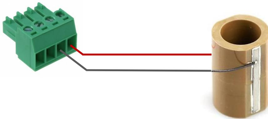
Bender actuators can be driven with a single bias voltage, for example 200 V, or a bipolar bias voltage, for example  $\pm 100$  V. The  $\pm 100$  V bipolar configuration is shown below.
