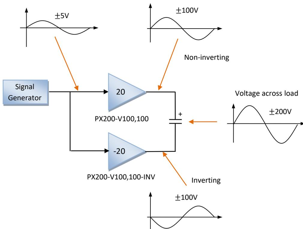
Figure 5. Bridge mode configuration for obtaining  $\pm 200\text{V}$
