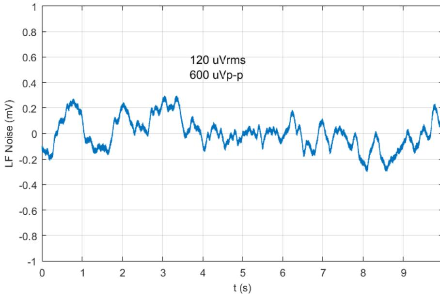
**Figure 4. Low frequency noise from 0.03 Hz to 20 Hz**
