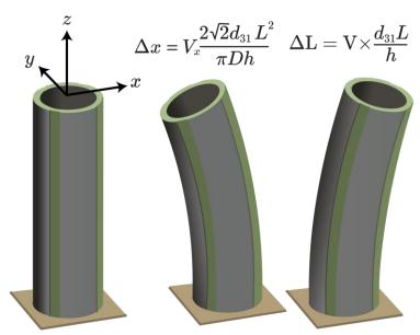
Figure 10. Piezoelectric tube with a fixed base and free end (full details)
