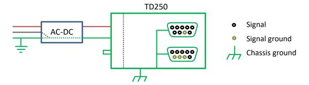
Figure 3. TD250 Chassis and signal ground configuration
