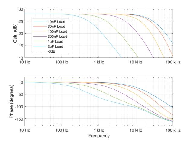
Figure 7. Small signal frequency response for a range of load capacitances
