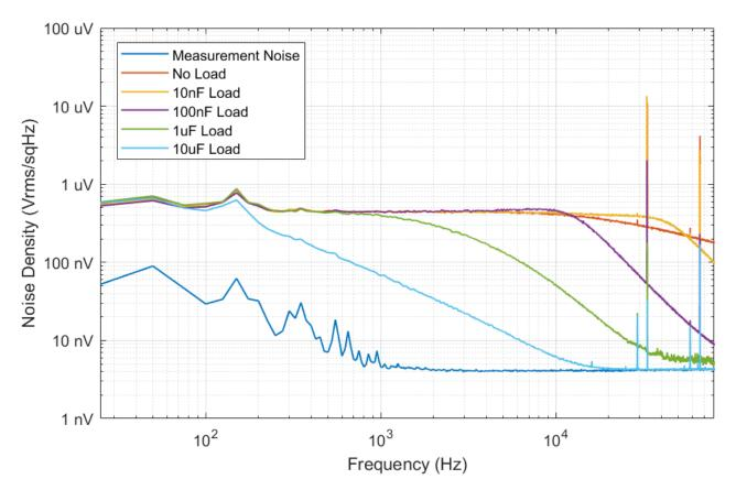
Figure 8. Output noise density for a range of load conditions in  $Vrms/\sqrt{Hz}$
