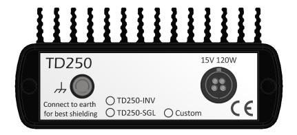
The rear panel includes a chassis earth connector that can be used to improve shielding, particularly when using an alternative power supply with an isolated output. This connector will accept a wire lug, 4mm plug, or stripped wire. The negative terminal of the power input connector is also connected to the chassis. Since the negative output terminal of the included power supply is connected to earth, the chassis is normally earthed.
