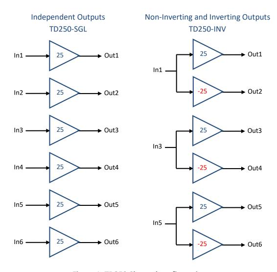
Figure 1. TD250 Channel configurations
