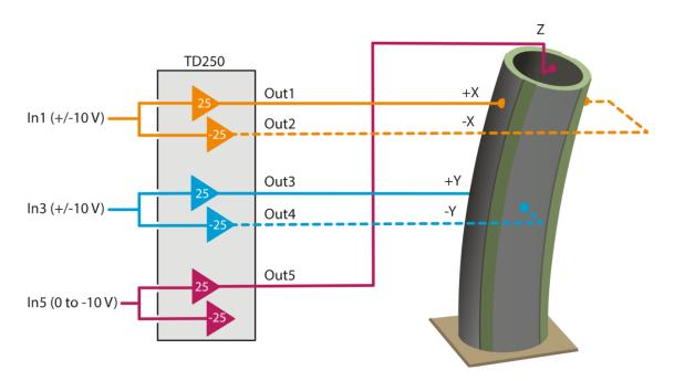
Figure 11. Driving piezoelectric tubes with the TD250-INV (driven internal electrode configuration)
