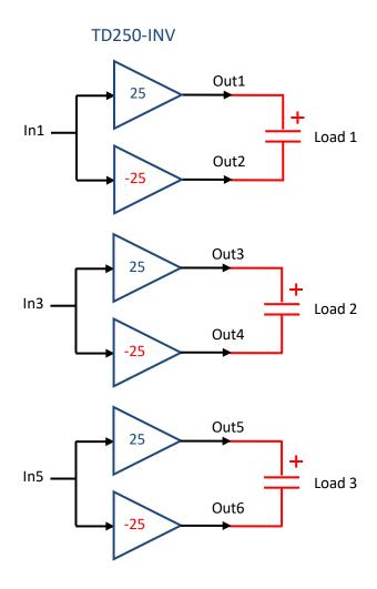
Figure 12. Bridged load configuration for obtaining +/-500V.
