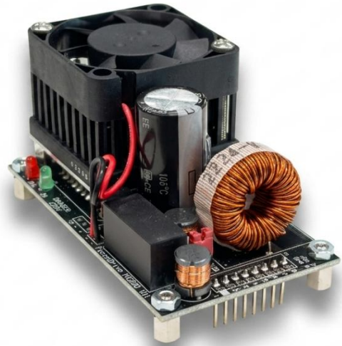
Figure 111. PCB Mounting version where the screw terminals are replaced by pin headers.
